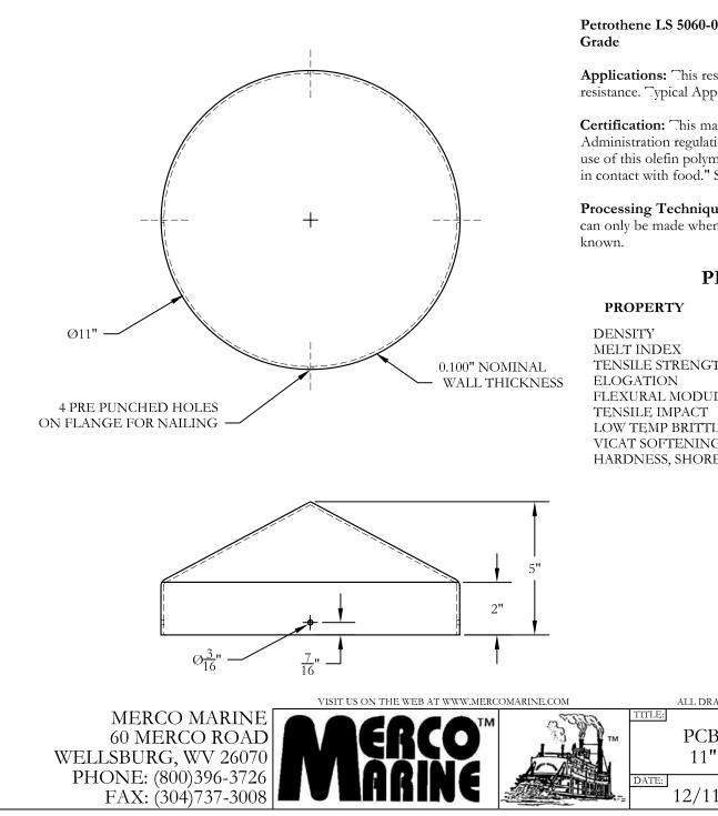
Petrothene LS 5060-00: High Density Polyethylene Injection Molding Grade
