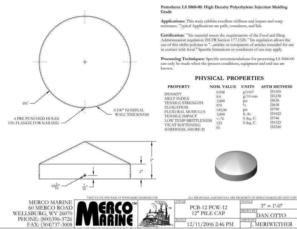
Petrothene LS 5060-00: High Density Polyethylene Injection Molding
